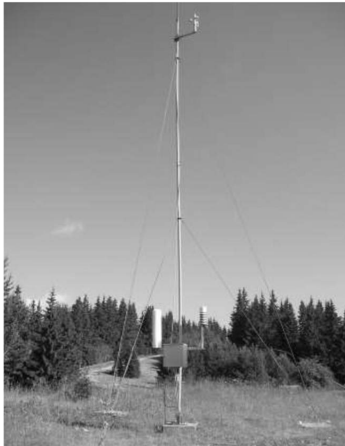
Figure 4: Mast LMS Rozhen - Gamma probe and Meteo
