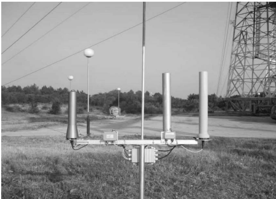
Figure 5: Picture of a renewed sensors LMS. At left is spectrometric probe in the middle is the start and to the right is the new dosimetric probe.
